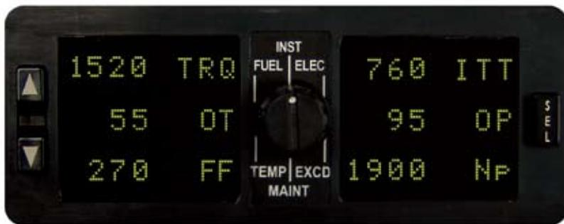
The Blackhawk Precision Hawkeye DigiLog Gauges can be teamed up with the optional Digital Display Monitoring Panel (DDMP) to provide downloadable exceedance recording, storage and playback.
