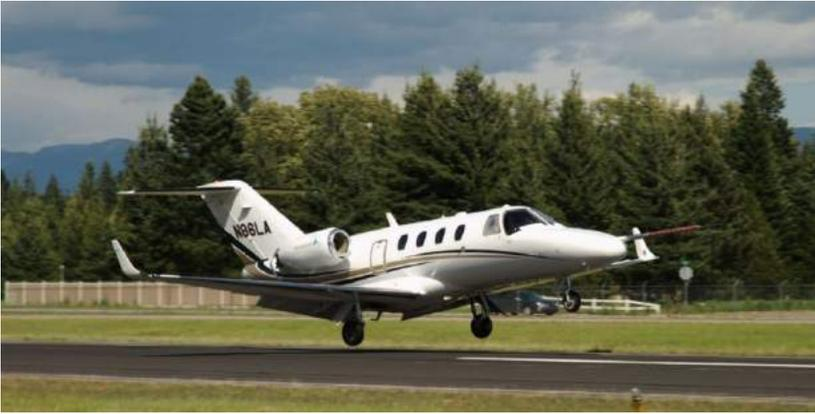
"As a professional pilot, I must say that TAG's winglet- equipped CJ was impressive from takeoff at MTOW, to touchdown. The noticeably improved climb performance experienced through the flight levels is a testament to the success and effectiveness of Tamarack's winglet technology. Fuel consumption to top of climb (TOC) at FL410 was only 560 lb (82 gallons) and just under 35 minutes, which is a big advantage over the winglet-less platform.
